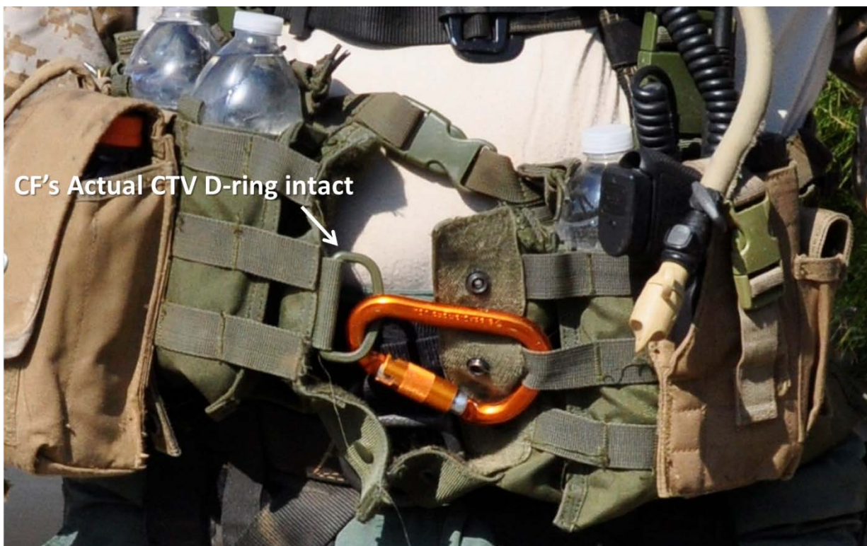
Figure 4.4. CF CTV D-ring intact, close-up, taken 2 days prior to mishap (Tab Z-6)
